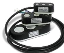
The new **MC3** measurement system comprises three efficient transformers in a single enclosure. The reduced size makes it a simple, efficient innovative system for measuring current by phases. It offers significant advantages during the installation phase of power analyzers in modular panels. Available in 63, 125 and 250 A versions, in accordance with the **IEC 60044-1** transformer standard.
