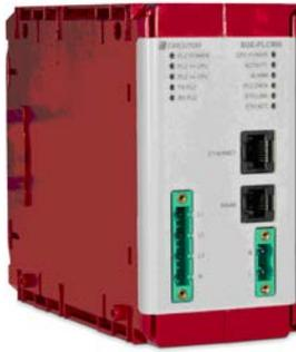
The DCSK SGE.-PLC800 Concentrator is the unit that manages and reads the three-phase and single-phase energy meters with DCSK communications connected directly to the low voltage network. The format used is of the DIN rail type with PLC DCSK communications, Ethernet port and RS-485.
