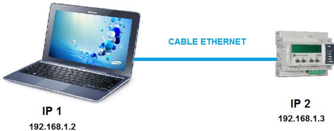
Figure 1: Configuration of a static IP.
