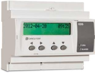
**EDS (Efficiency Data Server)** is an *energy efficiency manager*. The device has an RS-485 communications bus, as well as 8 digital inputs and 6 digital outputs via relay, which allow it to communicate with external field devices, representing and storing the information via its Ethernet connection and integrated web server. **EDS** also has a standard XML server, through which other external applications can integrate information from the device easily and intuitively.
