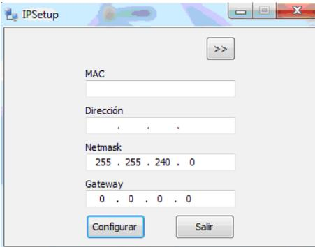
In the field "**MAC**" it must be typed the physical address of the unit using scripts as separator, this data is showed on to the lateral label of the equipment and the format is 14:A6:2C:XX:XX:XX.
