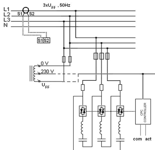
Fig. 5-1.- Auxiliary supply by means of autotransformer
