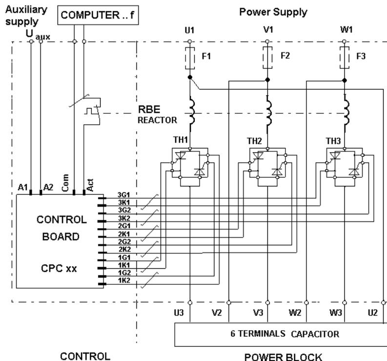
Fig. 4-4 .- Basic connection diagram of the **CPCxx** to the power block
