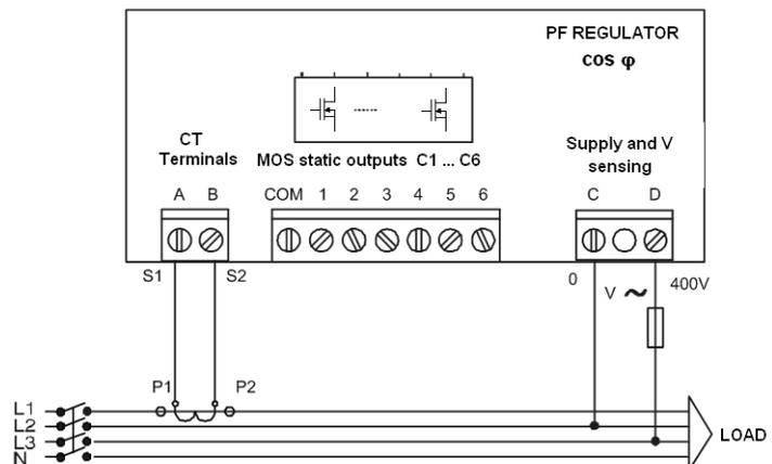
Fig. 6-2 .- Standard connection of a regulator with a single CT (3 current transformers will be used when Computer + is used. See the specific manual of the Computer + regulator)
