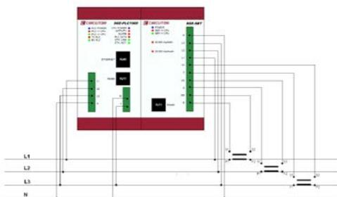
Connection diagram of the SG-PLC1000/50 concentrator and SGE-SBT supervisor module
