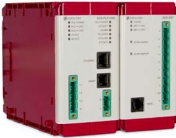
The PRIME **SGE-PLC1000** and **SGE-PLC50** concentrators manage and read single and three-phase energy meters with PRIME communications systems connected to the same low voltage network. The format used is of the DIN rail type with PLC PRIME communications, Ethernet port and RS-485 or RS-232. The concentrator can add an indirect three-phase meter, with the same format and LV supervision functions (**SGE-SBT**).
