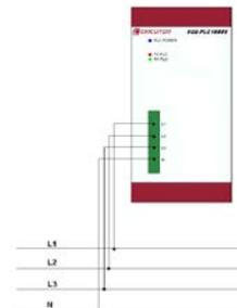
Connection diagram of the SG-PLC1000S concentrator
