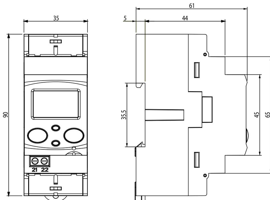
Figure 13: Dimensions of the CEM-C10.
