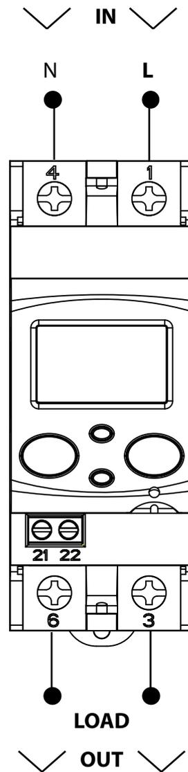
Figure 2: Connection diagram, CEM-C10.
