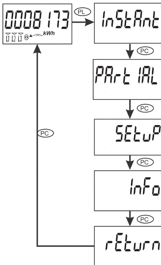
Figure 7: Navigation diagram in reading mode of the CEM-C10.
