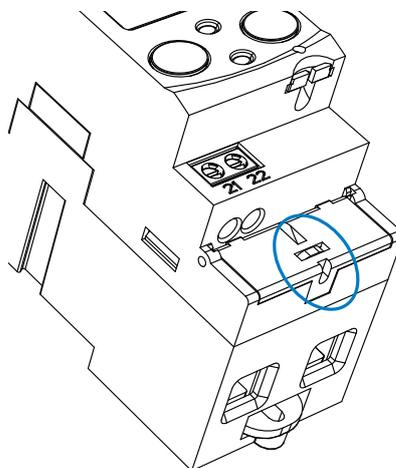
Figure 4: Seal of the CEM-C10.
