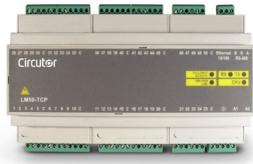
The **LM50-TCP+** is an instrument equipped with 50 voltage-free digital inputs. Through these inputs, using a master communications software, the user can detect the logical state of the inputs (open or closed contact), or otherwise know the number of impulses or manoeuvres received by an outside impulses emitter (energy, water, gas meter, etc). The recorded parameters are shown in the following variables table (see section 2.3.-).
